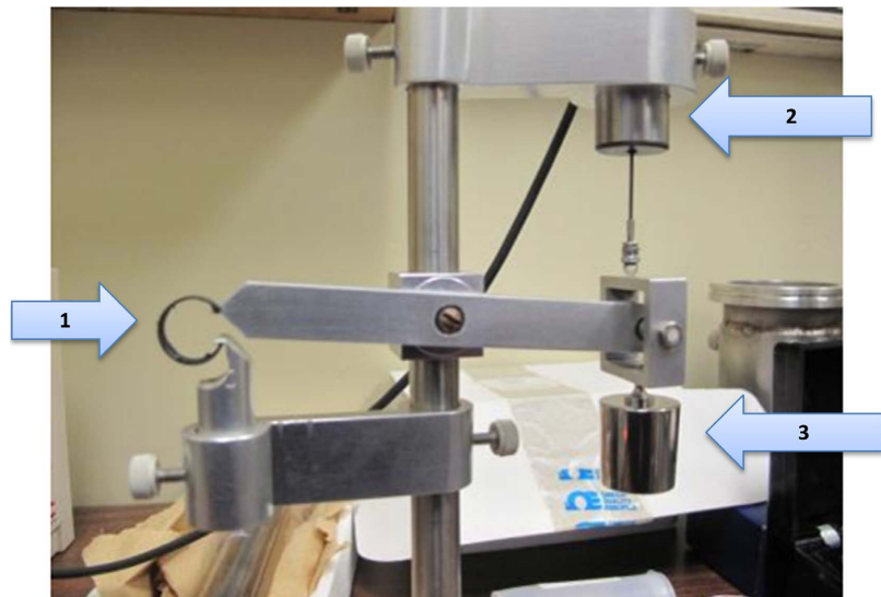
Figure 1. Deflection of slotted C-ring in a Class-1 precision lever system subject to 100.00 \pm 0.01 g mass-load force [61]. C-ring (1), Linear displacement transducer (2), 100 g weight (3).
