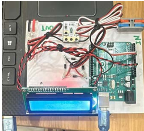
Figure 3. Electronic Circuit to display the value of power generation.
