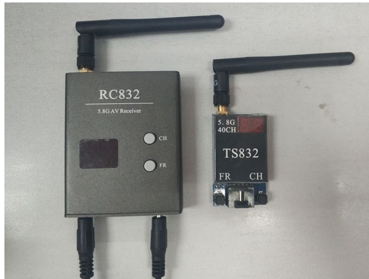
Figure 6. Physical components of the transmitter and receiver.
