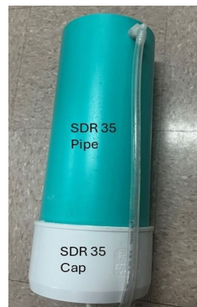
Figure 1. The main body and end cap of a novel Artemia feeder.
