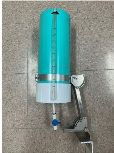
Figure 7. Novel Artemia feeder connected to an Arvotech TD 2000 mounting assembly.
