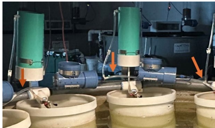
Figure 4. Artemia feeders connected by a common airline (note orange arrows).
