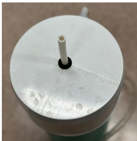
Figure 5. Uniseal and PEX tubing at the bottom end of a novel Artemia feeder.
