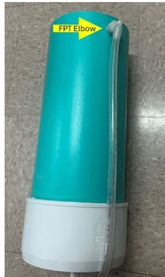
Figure 3. The outside air delivery system for a novel Artemia feeder.
