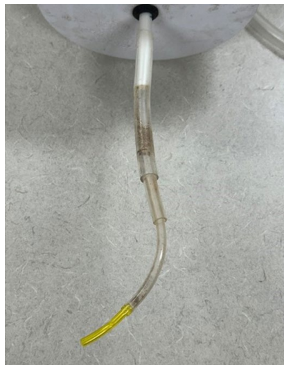
Figure 9. Retrofit of an Artemia feeder showing the decreasing diameters of vinyl tubing.
