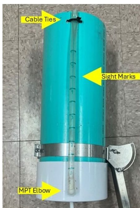
Figure 6. View tube with graduation marks on the outside of a novel Artemia feeder.
