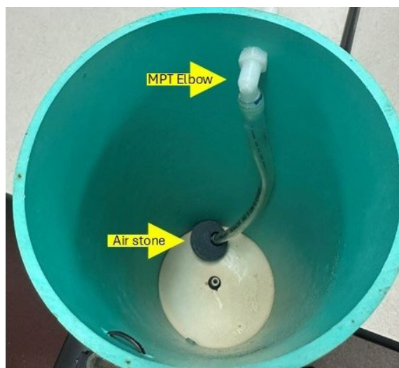
Figure 2. The inner air delivery system for a novel Artemia feeder.
