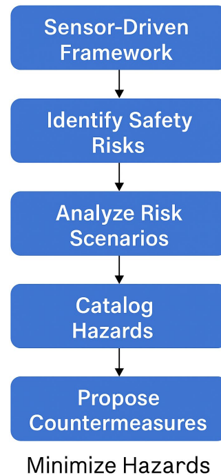
Figure 6. Sensor-driven workflow for AGV hazard identification and mitigation.
