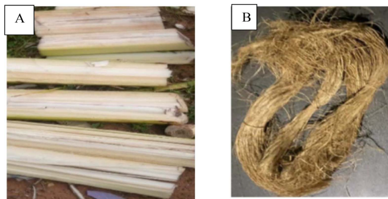
Figure 1. Fiber's extraction process: (A) banana stem lamella; (B) banana fibers maintaining the Integrity of the Specifications.
