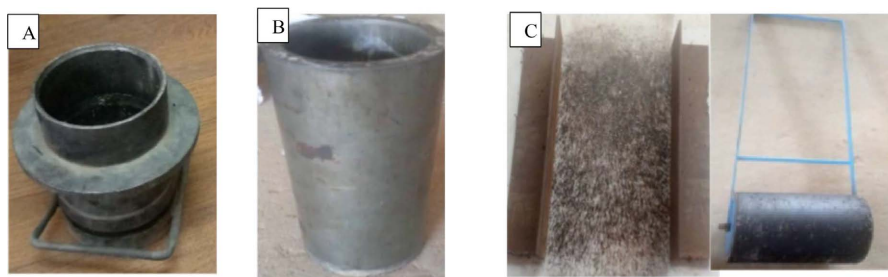
Figure 3. Shaping molds: (A) Marshall mold, (B) Duriez mold, (C) Prismatic specimen shaping device.
