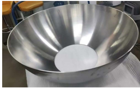
Figure 7. The product of large-diameter thin-walled titanium alloy shell.
