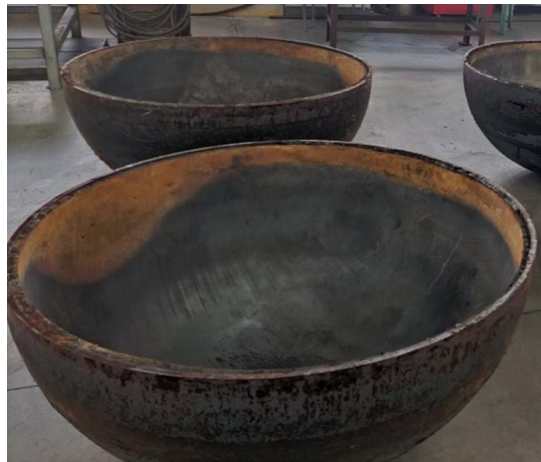
Figure 6. Experimentally produced titanium alloy shell.
