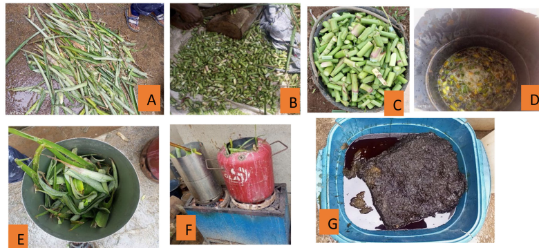
Figure 4. (A) preparation of PLF; (B) preparation of EGSF; (C) 4 kg of chopped EGSF; (D) Chopped EGSF + 4% Caustic Soda + HO 2 ; (E) 4 kg of PLF + 4% Caustic Soda + HO 2 ; (F) Pot on red hot charcoal for cooking; (G) Digested Pulp mixed with black liquor.
