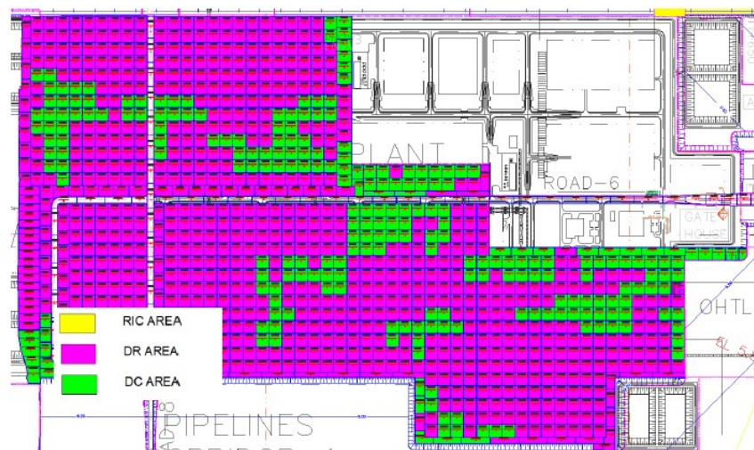
Figure 5. Early work screening of a segment on site with pre-CPT boxes [23].
