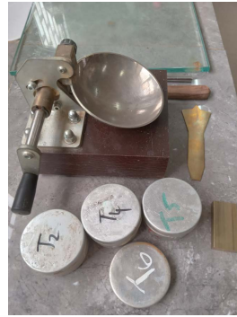
Figure 7. Equipment for Atterberg limits.
