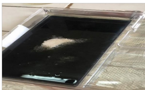
Figure 6. Illustration of PS dissolution in d-limonene after 20 s.
