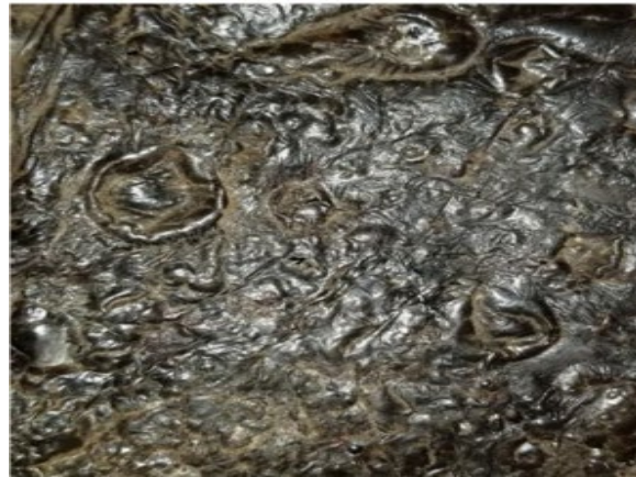
Figure 8. Appearance of polystyrene after molding seen from above.
