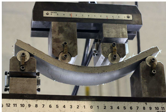
Photo 17. ECC bendable concrete in flexural test machine.
