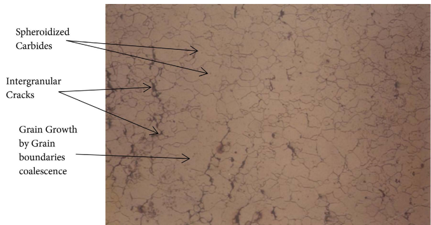
Figure 9. Micrograph of A2 at 200× magnification. No Pearlites were seen.
