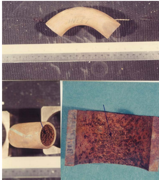
Figure 5. Superheater Inlet Elbow. Obvious corrosion products were seen on the internal surface (arrowed example).
