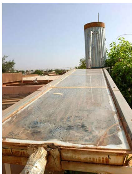
Figure 1. Prototype of SWH studied.
