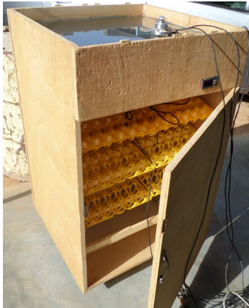
Figure 1. Image of the incubator fitted with a flat-plate collector.
