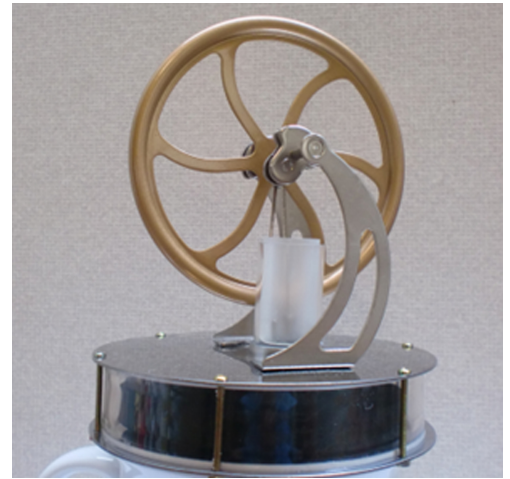
Figure 2: A low temperature Stirling engine (LTSE) works with heat flows (entropy flows), creating nonequilibrium irreversible states (NISs).
