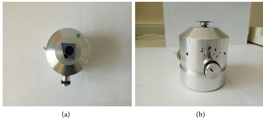
Figure 3. (a) and (b) External views of the detector from the top (green LED is visible) and from the side of the mode switch selector. In its initial position, shown in the photo, the input of the amplifier is grounded to the cage. It often happens that operators, as well as ordinary people, accidentally accumulate a charge that “goes” to foreign objects with a spark discharge. When the sample holder in the mushroom shape (a standard disc has a diameter of 12 mm) is inserted into the site hole, the input stage may be damaged. On the left side is the power on switch.
