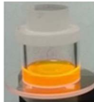
Figure 2. Photo of the cylindrical cuvette with R6G alcohol solution.
