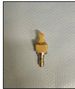
Figure 7. Post-milling inspection of crown.
