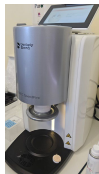
Figure 8. High-speed sintering and glazing of the zirconia crown in CEREC SpeedFire furnace.
