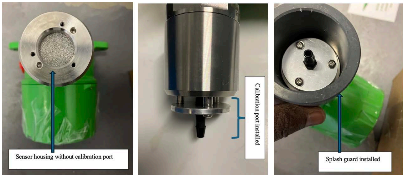
Figure 8. Geometry around the sensor when the splash guard is inserted.
