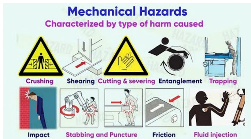
Figure 5. Mechanical hazards. Source: WorkSafeVP (2023) [31].
