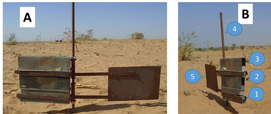
Figure 4. A three BSNE mast installed in the Bangou Koiré millet field: A. side view; B. front view: 1, 2, and 3 are respectively BSNE at the bottom, middle, and high levels above the soil; 4: mast; 5: weathervane.
