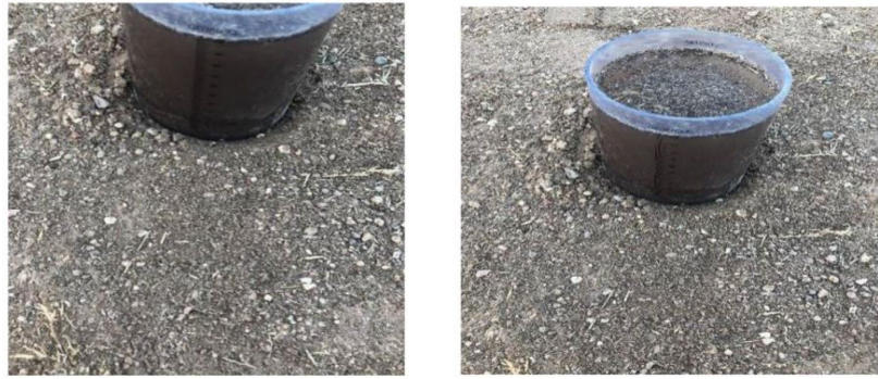
Figure 2. The double ring infiltrometer. Source: Fieldwork. Infiltrometer showing ongoing infiltration measurement.
