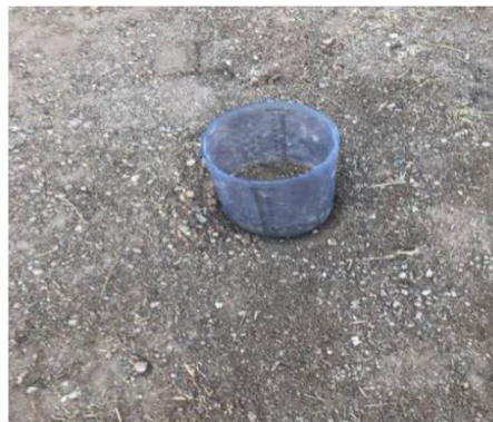
Figure 1. The double ring infiltrometer. Source: Fieldwork. Infiltrometer cylinder filled with water, showing initial fill level.
