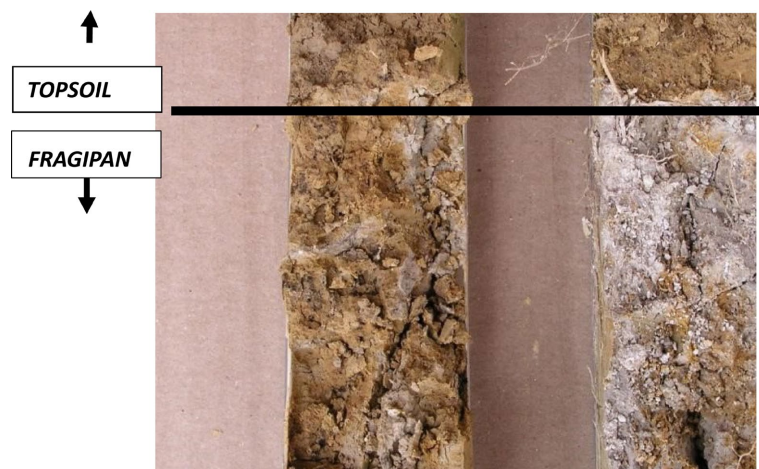
Figure 2. Visual signs of fragipan degradation by ARG + NaF (right core), compared with untreated fragipan (left core).
