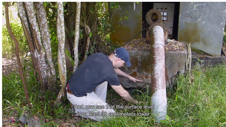
Figure 15. Evidence of subsidence. The land surface has dropped 45 cm. Published with permission of the Editor of Open Journal of Soil Science.
