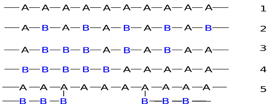
Figure 1. Different types of polymers: 1) homopolymer 2) alternating copolymer 3) random copolymer 4) block copolymer 5) graft copolymer.
