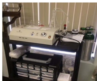
Figure 1. Quantum 5 ozone generator connected to an oxygen tank.
