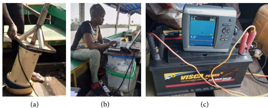
Plate 1. Views of the ADCP (a) et (b) and Garmin 521s echosounder (c) deployed on the Ouémé River and Nokoué lake (July 2022).
