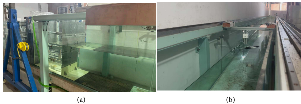
Figure 6. The environment of wave tank experiment (a) Multi-plate wave maker; (b) Model and wave probe settings.
