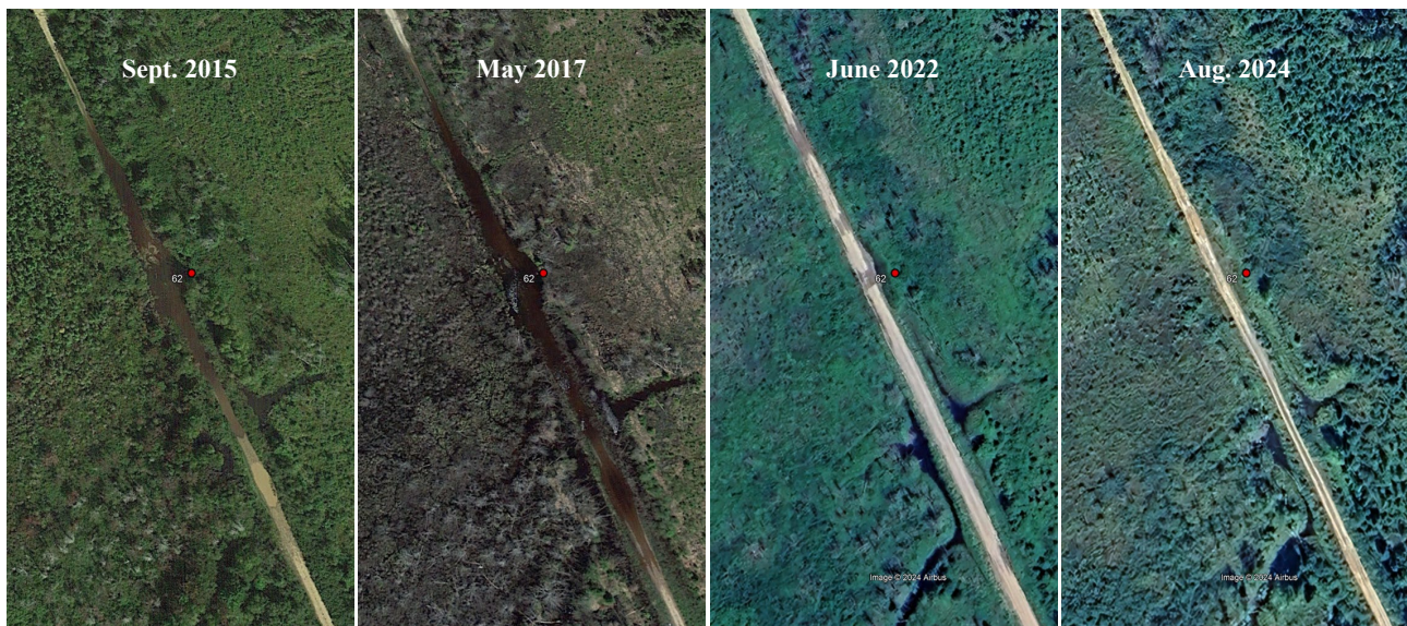
Figure 2. Best-focused historical Google Earth images centered on road flooding (Location 62) along the Aboujagane Road before (Sept. 2015, May 2017) and after (June 2022, Aug. 2024) road repair, centered on Location 62.
