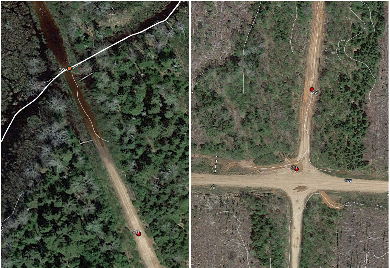
Figure 4. Road deterioration examples. Left panel: FA > 4 ha channel-induced flooding (f) at Location 39; FA > 0.1 ha channel-induced rutting (r) at Location 40. Right panel: FA > 0.1 ha channel-induced braiding (b) and puddling (p) at Locations 22 and 23, respectively. Thin and thick white lines: DEM-derived flow channels > 0.1 ha and > 4 ha.
