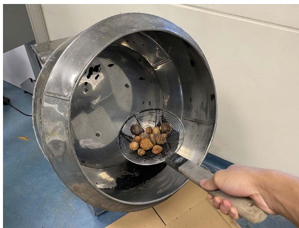
Figure S1. Model YX-65 Sweet rice ball forming machine used to create biochar seed balls for L. corneus , C. myrsinifolia and E. sylvestris .
