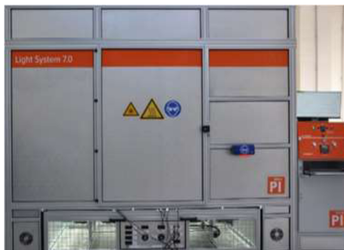
Figure 10. PV module electrical stabilization system.
