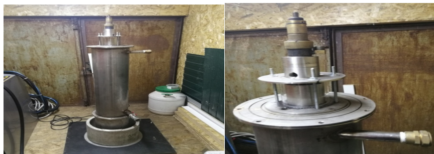
Figure 6. General view of the plasma-chemical reactor of the mobile unit “Plazmon-3” for the treatment of solid medical waste with a plasma generator PUN-1 installed on it.
