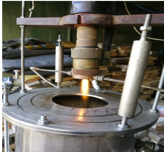
Figure 3. General view of the PUN-1 plasma generator. Plasma generator is modeled on a plasma-chemical reactor for the utilization of solid HLW.
