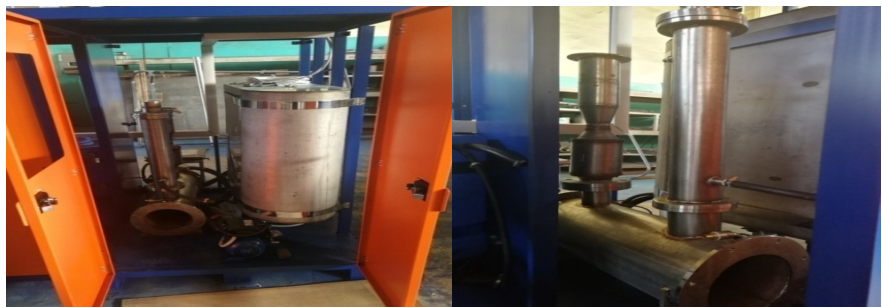
Figure 4. General view of the plasma-chemical reactor of the Plasmon-2 mobile unit for liquid medical waste treatment.
