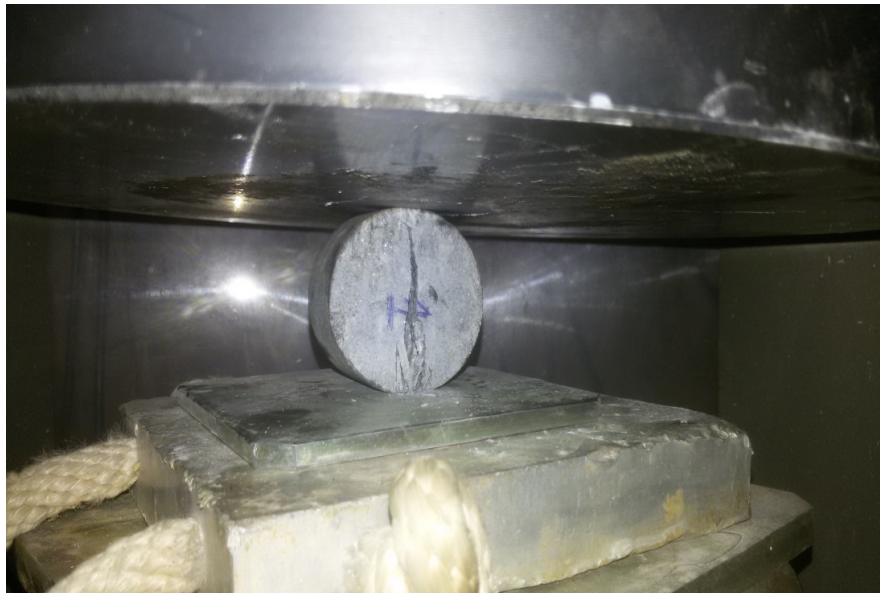
Figure 5. Loading of core sample for tensile test (UTS).
