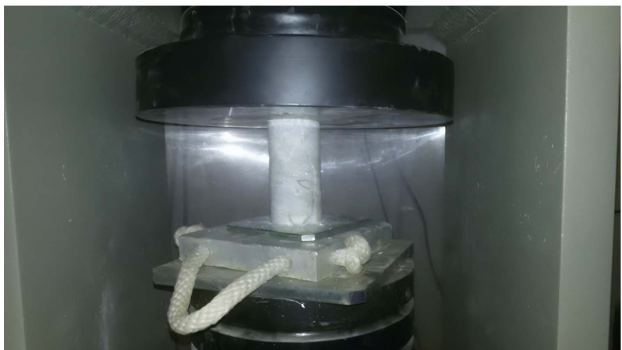
Figure 4. Loading of core sample for compressive test UCS.
