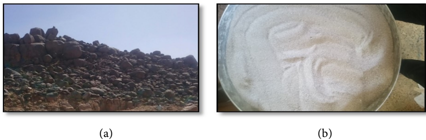
Figure 2. (a) Illustrating the granite stone before its fracture, (b) Illustrating the granite stone after its fracture and grinding.
