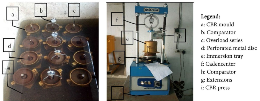
Figure 8. Equipment for determining the CBR load-bearing index
