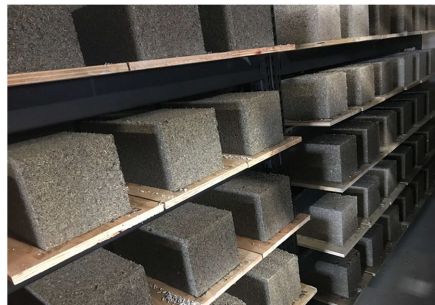
(a) Hempcrete block cast and cure under strict standards and environments
