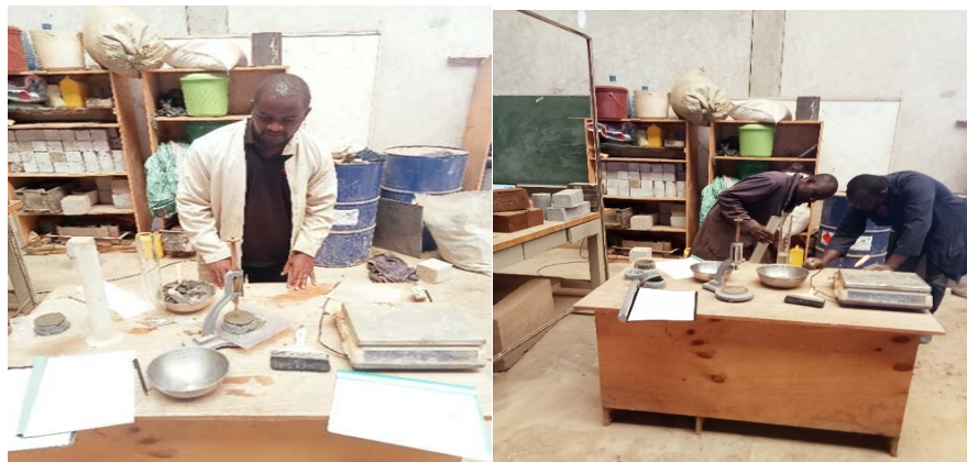
Figure 3. Ongoing setting time test at JKUAT materials laboratory.
