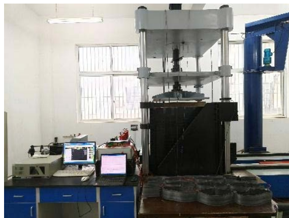
Figure 2. DW1280L multi-channel large electro-hydraulic servo direct shear pull-out tester.
