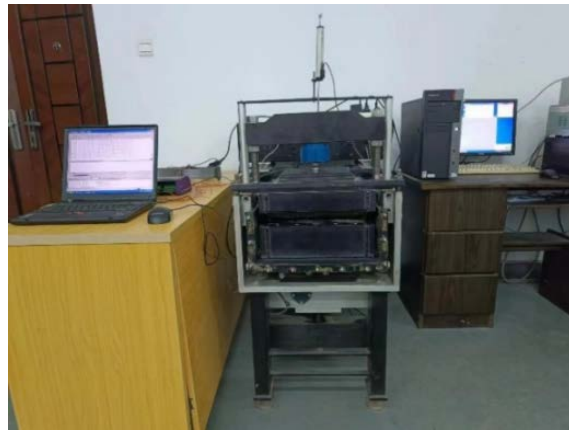
Figure 1. Geocomp shear Trac-II automatic straight shear instrument.
