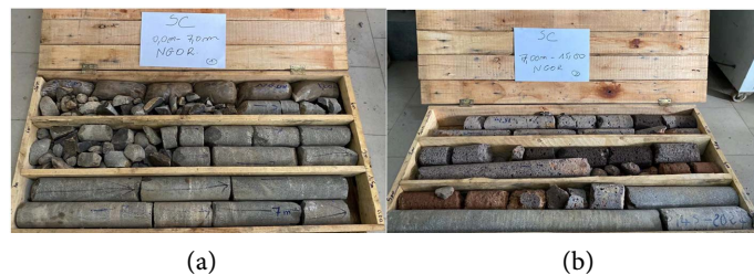
Figure 3. Intact rock cores in core box collected between 0.0 and 20.0 m.
