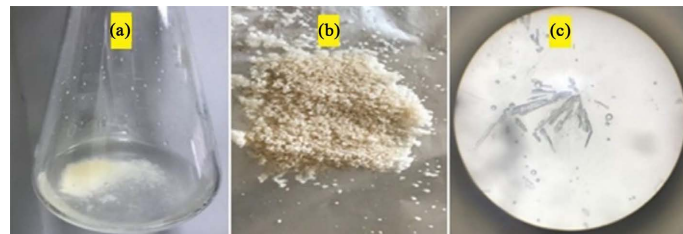
Figure 7. Bio-cement produced by S. epidermidis EDH (a), after being dried at 105°C overnight (b), and the resulting bio-cement crystals observed under light microscopy (c) [21].
