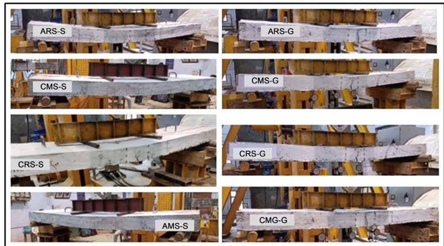
Figure 6. Deflected profiles of slabs.
