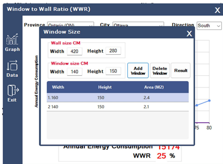
Figure 8. Input data for wall and windows dimensions.
