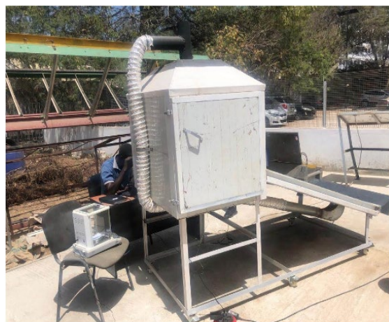
Figure 1. Indirect solar dryer with forced convection.
