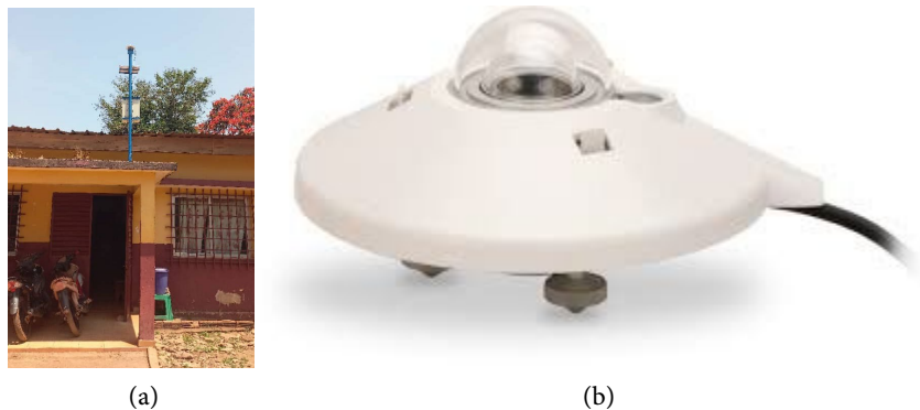
Figure 2. View of the solar irradiance measurement equipment system installed on the roof of a building at the University of Kankan. (a) Solar irradiance measurement equipment installed on site; (b) Pyranometer.
