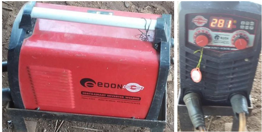
Figure 10. Electric arc welding station with coated electrode.
