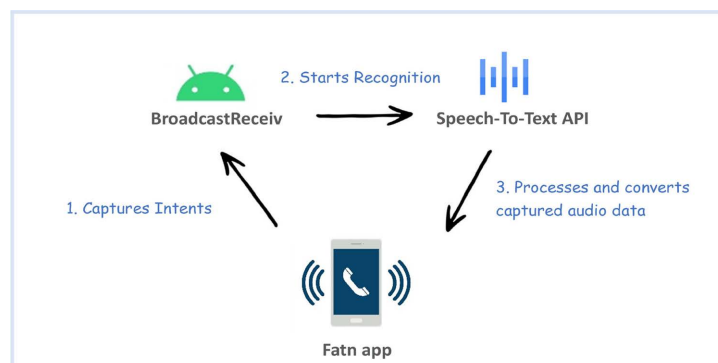
Figure 5. Model architecture for speech recognition technology.
