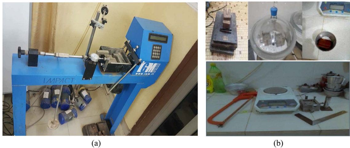
Figure 11. Direct shear test equipment. (a) shear press; (b) Accessoires.
