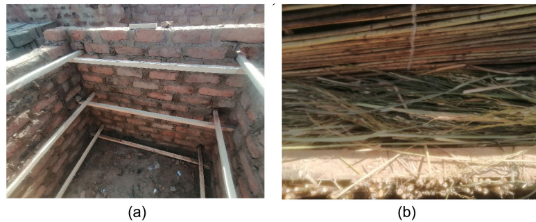
Figure 4. (a) Cladding for insulation; (b) Rice straw placed between reed mats (sample 2).
