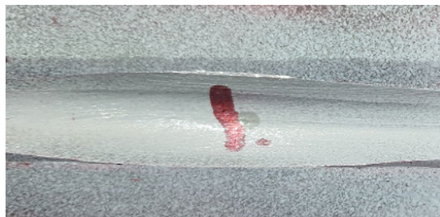
Figure 4. A colored or fluorescent dye is applied to the surface, penetrating open cracks. Excess dye is removed, and a developer highlights the cracks.
